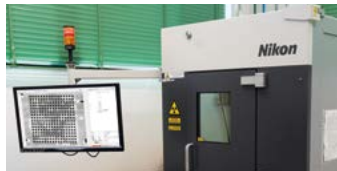
X-ray inspection of electronic boards and components
