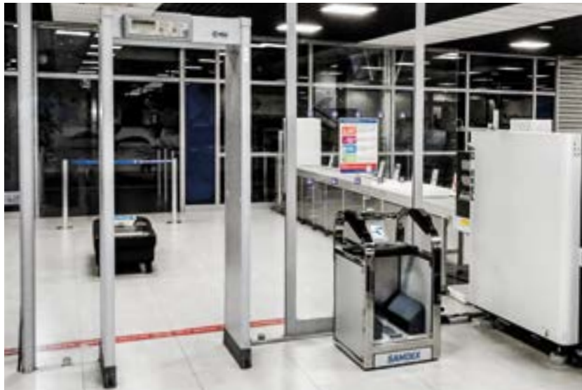
SAMDEX® (Shoes Metal & Explosive Detector) STAC certified, DfT approved, BPOL certified, NCTV certified Is the first equipment with double technology for the simultaneous detection of metallic and explosive threats concealed in shoes without the need of divesting shoes.
